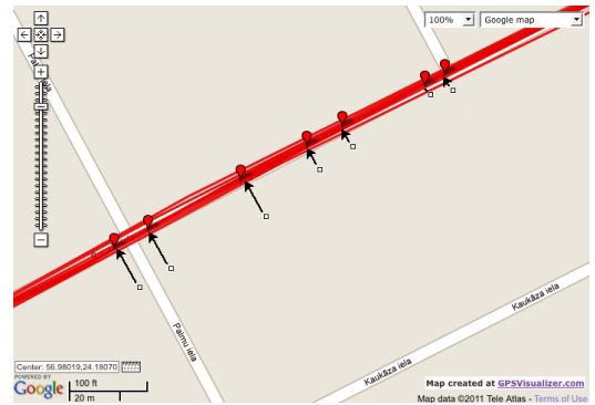
Figure 3. Manually marked ground-truth position improvement, by calculating perpendiculars to the test drive trajectory
