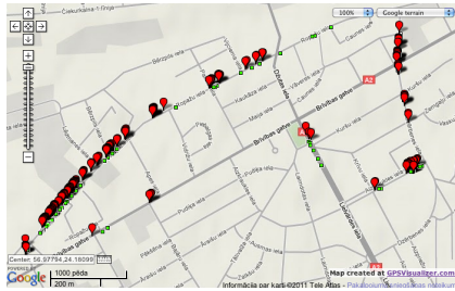
(a) Android (red balloons) and our previous methodology (green) [6] detected potholes, GPSVisualizer.com used
